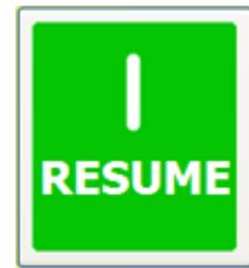
The button in this state has exactly the same effect as the button in the Start state, but is shown if an operation has been interrupted by a warning or by the Stop button.
